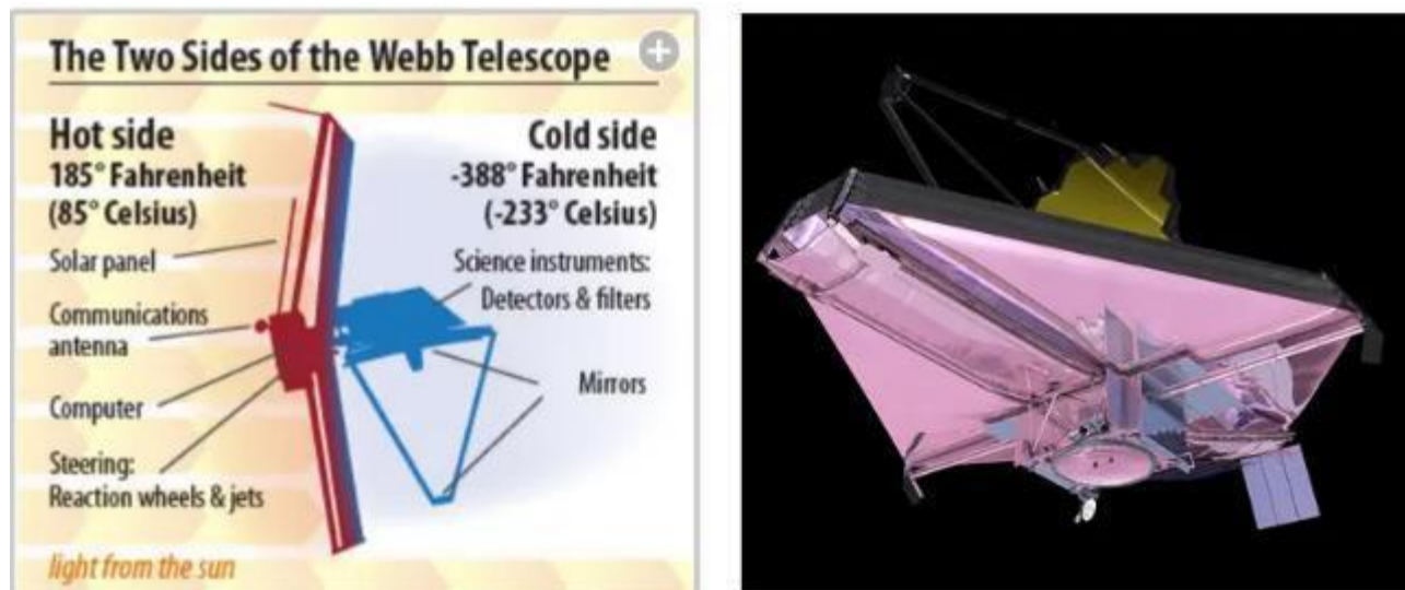
Fig 5: The two sides of the Webb telescope (left). The 'hot' side of JWST with the sunshield protecting the main optics from sunlight (right).
